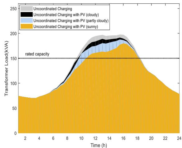
Fig. 6. Transformer load with uncoordinated charging and PV.
