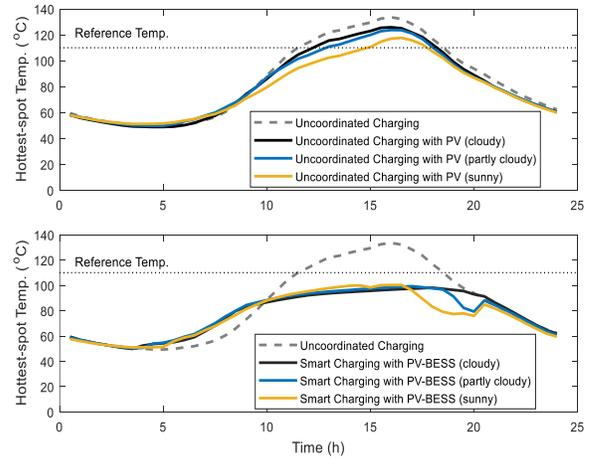
Fig. 9. Transformer hottest-spot temperature to all scenarios.
