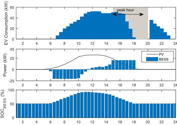
Fig. 8. EV consumption, PV and BESS operation on a sunny day in summer.
