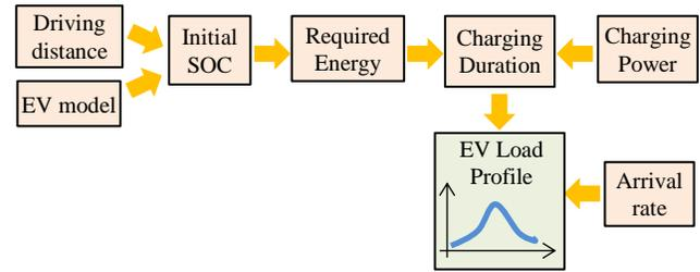
Fig. 4. Flowchart for EV load profile evaluation.
