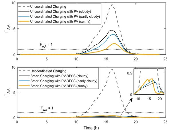
Fig. 10. Transformer accelerated aging factor  $F_{AA}$  to all scenarios.
