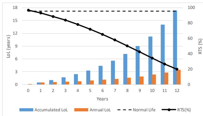
Fig. 11. Transformer RTS and used life over the years.
