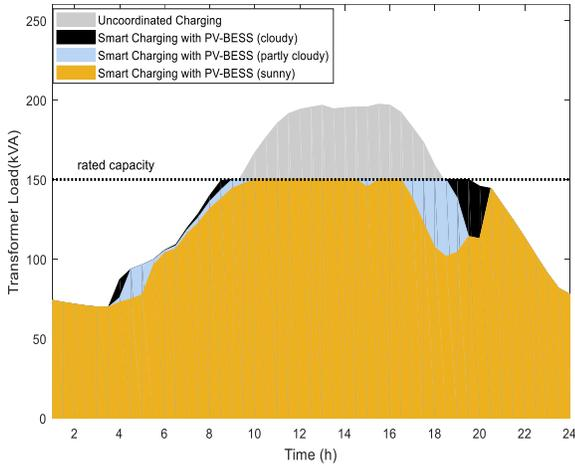
Fig. 7. Transformer load with smart charging and PV-BESS.
