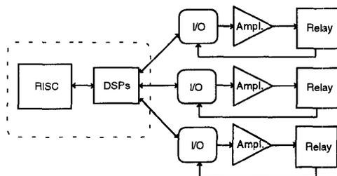
Fig. 2. Real-Time Simulator Architecture
